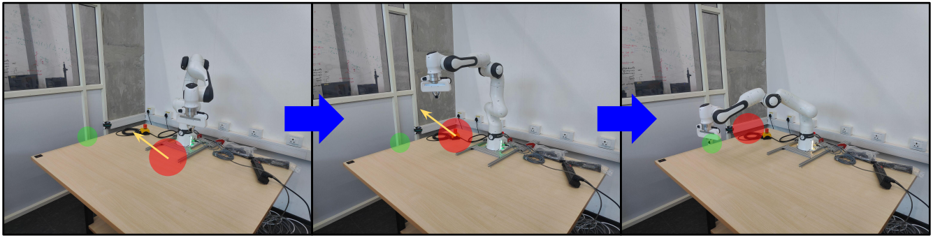
Fig. 5: The figure illustrates the Franka Panda manipulator advancing toward its designated target while executing collision avoidance maneuvers in the presence of a dynamic obstacle. The green region denotes the goal area , and the red circle identifies the moving obstacle , with its direction indicated by the arrow.
